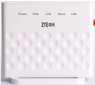
Figure 3-1 Indicators of the ZXHN F601 unit
